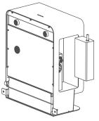
If you need to add cleaning solution, please take out the cleaning solution container, pour the cleaning solution and put it back into the workstation .(as shown below)
