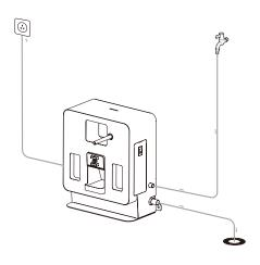
• Put the CC1 robot charging adapter (not in the workstation package) purchased earlier into the workstation(\*When installing, pay attention to the heat dissipation hole of the power adapter facing down).
